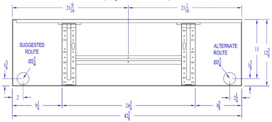
The holes shown are the best locations to route the refrigerant lines, condensate drain, and electric. For installations where the line set will be accessible on the backside of the wall, use the alternate route. When the line set will be run inside the wall before the drywall is installed, use the suggested route. This will leave the flare connections exposed so they can be connected after the walls are finished.
