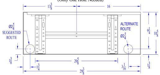
The holes shown are the best locations to route the refrigerant lines, condensate drain, and electric. For installations where the line set will be accessible on the backside of the wall, use the alternate route. When the line set will be run inside the wall before the drywall is installed, use the suggested route. This will leave the flare connections exposed so they can be connected after the walls are finished.
